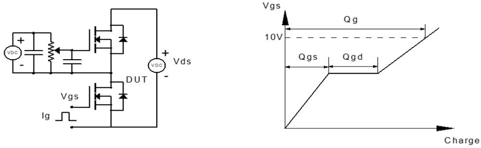
Figure 1: Gate Charge Test Circuit & Waveform
